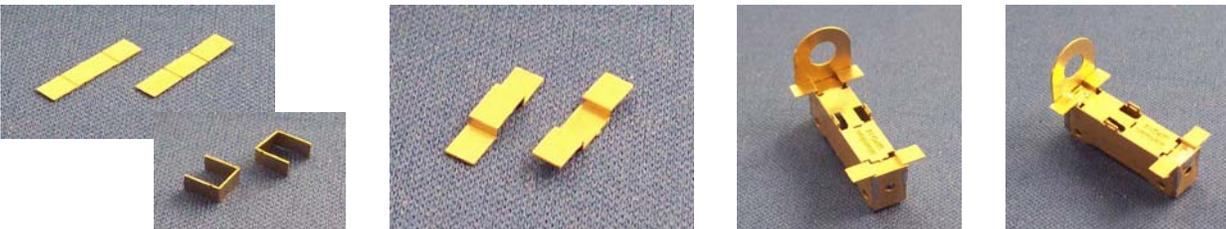
Remove the two cross pieces A4 from the fret. Fold the four half etched lines on each piece with the half etch on the inside. Fit at each end in the open areas of the frames. Solder in place.
