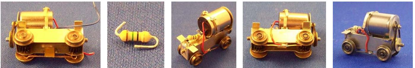
Shape and cut the two ends of the phosphor bronze strip to rub against the back of the insulated wheels.
