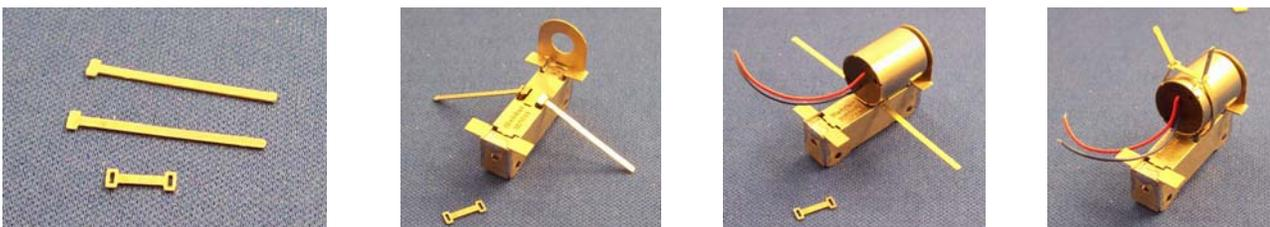
Remove the two long straps A5 and short strap A6 from the fret. Fit one of the long straps through each of the slots in the frames as shown. Position the motor and fit the short strap between the two long straps. Tighten but do not solder.
