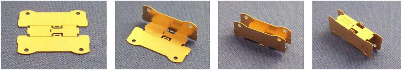
Remove the main frames A1 from the fret and fold the two sides with the half etched lines on the inside of the joins
