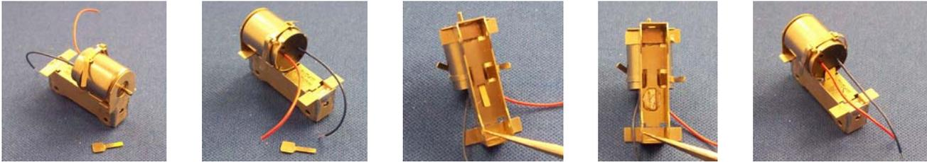
Remove the motor stop A7 from the fret. Fit through the slot in the top of the frames with the broad section outside. Bend and solder in place inside the frames.
