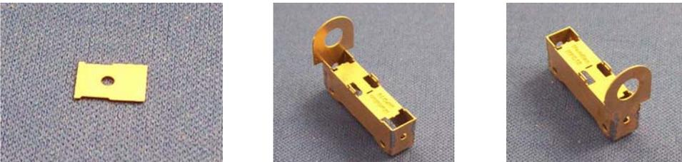
Remove the other end spacer A3 from the fret and fit between the two sides noting the interlocking steps in the pieces to set position. Solder in place.
