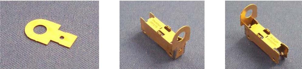
Remove the motor end spacer A2 from the fret and fit between the two sides noting the interlocking steps in the pieces to set position. The motor end spacer goes at the opposite end to the 'Meridian' etched name on the frames. Solder in place.
