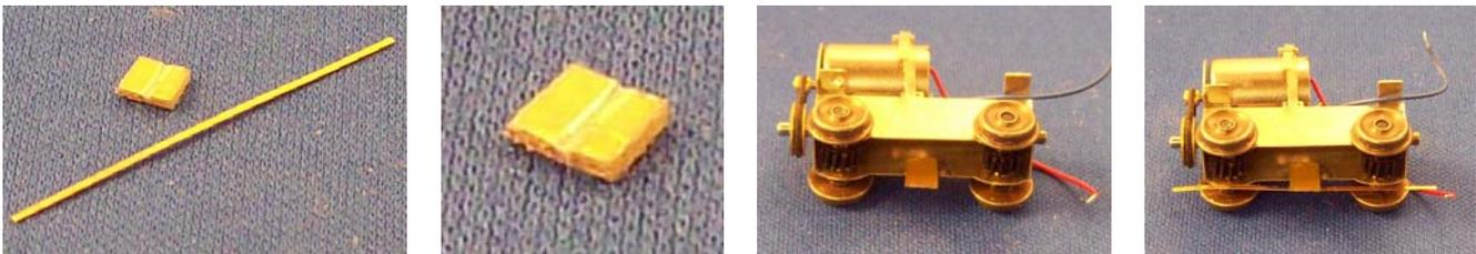
Locate the PCB material L and phosphor bronze strip M. Gap the PCB about 1mm from one edge. Solder the copper side to the inside of the frame on the side which has the insulated wheels fitted so that the 1mm section and gap are below the edge of the frame. Solder the phosphor bronze strip to the lower 1mm section of the PCB so that it is insulated from the frame (no touching, no solder bridges).
