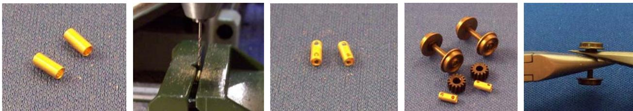
Locate the two shaft adapters E. Drill four 0.6mm holes in the ends of the adapters ideally using a mini drill in a drill stand or press. Alternatively a hand held mini drill or pin chuck can be used but the shaft adapter should be held in a vice and you may wish to file a flat on the end of each shaft adapter and only make one or two holes in this case. These holes are used for applying thread lock fluid to fix the adapters to the wheel sets.
