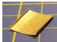
front and rear of the cab. Once you have achieved a good fit with a close joint to the top of the side solder or glue (using 5 minute epoxy) in place.
