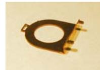
Remove the strap (B3) from the fret. Fit one end through the slot in the front and fold up or fold down and solder. Remove the back (B4) from the fret. Fold the item to 90° at the half etched line and then fold the two projecting tabs to 90° in the opposite direction. Trial fit the back to the base so that the two projecting tabs point down towards the base. Fit the slot at the top of the back into the strap. Check the cradle goes together neatly and adjust if necessary.
