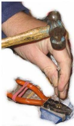
To remove the worm you need a pair of combination pliers/cutters, an elastic band, a vice (vise), a 1mm-1.5mm drift (e.g. old drill shaft or watchmaker's screwdriver) and a 4oz hammer. Take the Bachmann motor with the gear fitted and grip the motor shaft in the wire cutter section of
